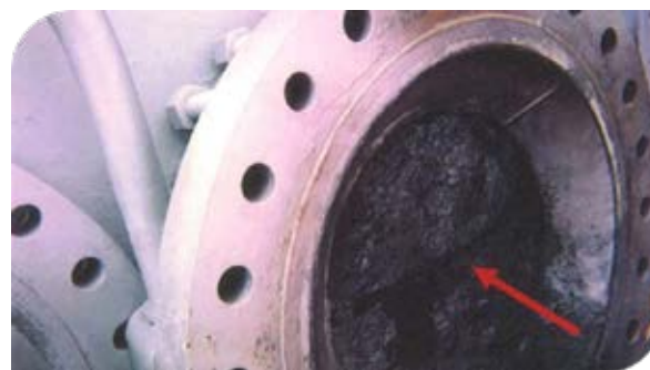
Figure 6 - coke deposition on the transfer line. source: FCCSA's archives
