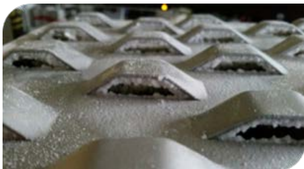
Figure 9 - Salt formation on trays. Source: Sulzer (3)
